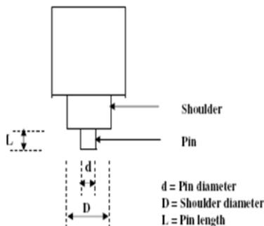
Schematic diagram of tool
